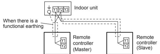
Group control and multiple wired remote control can be used together.
