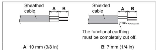
The functional earthing must be cut off. Failure to do so could cause a short to occur on the board, which could lead to damage, smoke, or even fire.
