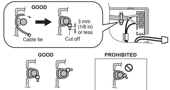
Install a cable tie in the direction as illustrated. Cut the end of the cable tie to the length as illustrated. Failure to do so may cause the end of the cable tie to press onto the board, which could cause damage.
