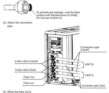
tightened properly by your hand, use a torque wrench to finally tighten it. Body side
