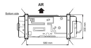
Fix securely with bolts on a solid block. (Use 4 sets of commercially available M10 bolt, nut and washer.)
