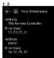
For the details of the indoor unit or outdoor unit error, refer to the error codes in each installation manual.
