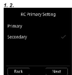
Set only one Primary remote controller. Units other than Primary are set to Secondary automatically. When remote controllers are set to "Secondary", setting items will be restricted.
