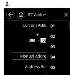
The address for this unit can be set from 1 to 32. However, do not set the same number as that for the remote controller address of an indoor unit connected using the same remote controller cable.
