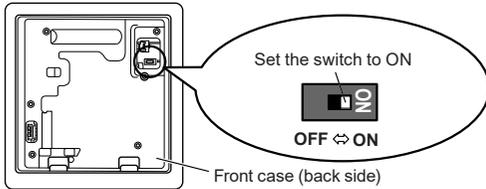
Before using this product, always set switch to "ON". If not set, when the main power is turned on again, the set data by menu operation will be erased and cause erroneous operation.
