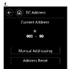
When the address is set manually, this mark \* is displayed. [001-01]
