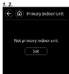
When changing the Primary Indoor Unit, another indoor unit cannot be made the primary indoor unit unless the settings of the current primary indoor unit are cancelled beforehand. ("Reset" cannot be performed while the indoor unit is operating.)
