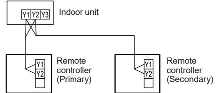
Group control and multiple remote control can be used together.
