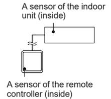
When the temperature sensor of remote controller is not used, the following functions cannot be used.
