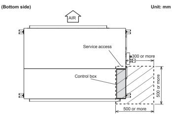
\* The service access necessary for fan units and filter maintenance.
