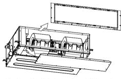
For the bottom air intake, position (1) the intake grille, and (2) the service panel, as shown in the following figure. (The factory setting is back air intake.)
