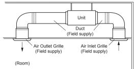
When connecting the duct, perform duct-insulation appropriate for the installing environment.
