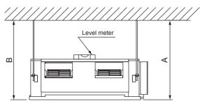
The side A of the unit with the drain port should be slightly lower than the opposite side B of the unit. The height difference between sides A and B should be from 0 to 20mm.
