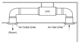
Be sure to install the air filter in the air inlet. If the air filter is not installed, the heat exchanger may be clogged and its performance may decrease.
