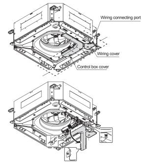
(2) Thread each cable through the holes or indents of the cabinet and connect the wires. (3) After wiring is complete, secure the cables with the cable clamps.
