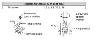
3.6.4. Wiring procedure Connection cable
