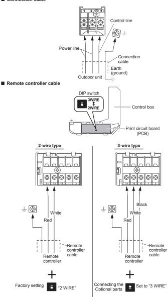
\*Earth (Ground) the remote controller if it has a earth (ground) wire.
