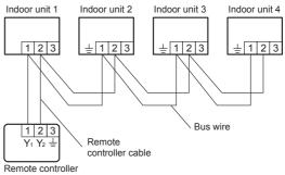
(2) Set the R.C. address (DIP switch setting) Set the R.C. address of each indoor unit using the DIP switch on the indoor unit circuit board.
