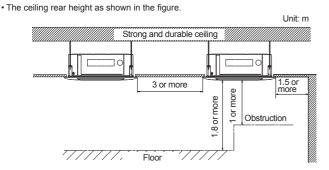
• This product can be installed at a height of up to 4.2 m. However, if the heights of the ceiling is higher than 3.2 m or lower than 2.7 m, it is necessary to set the position from remote controller. (Refer to "7. FUNCTION SETTING")
