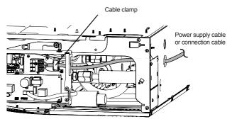
(4) Pass the remote controller cable through the knockout hole that you opened in the previous step, and fix the cable with the cable tie.
