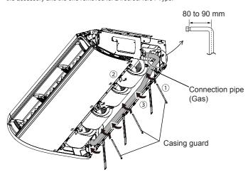
Finally, fix two positions using the screw removed in the previous step and the accessory tapping screw.
