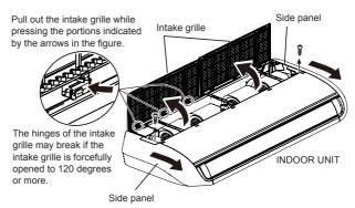
· Removing the casing guard
