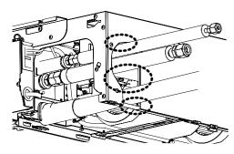
(2) Align three hooks of the side panel, and fix it to the backward. Then, fix it with the
