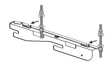
(3) Attach the unit body to the fixed suspension fittings, tighten two bolts on each side.
