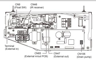
This air conditioner can be connected with the following optional kits. For details on how to install optional parts, refer to the installation manual included in each
