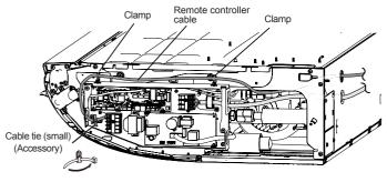
(5) Replace the Control box cover. Securely tighten the screws.
