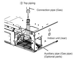
(5) For ④ Left rear piping and ⑤ Left piping , use the following procedure to install the connection pipe and attach the casing guard so that the fan motor and the casing do not contact the connection pipe.
