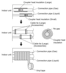
When using an auxiliary pipe, make sure that the cable tie used is insulated in the same way.
