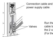
Run the connection cable and power supply cable to the rear of the outdoor unit between the 2 valves as shown in the figure
